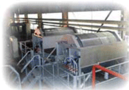
20 TPH LEAD SLAG SCREENING AT 200 MICRON, 70% OVERSIZE
