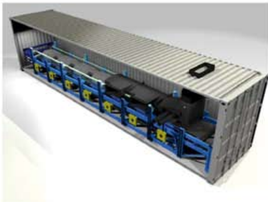
Phase 2: LaDePa showing the feed screws
